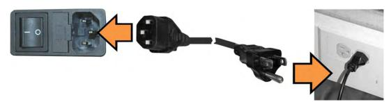
Figure 3-7. Apply AC Power to the Unit
