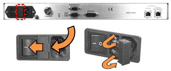
Figure 3-8. Replace the AC Fuses
