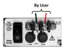
Figure 3-10. Apply DC Power to the Unit
